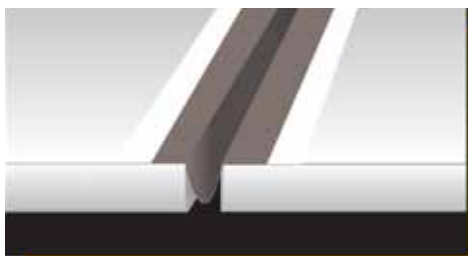
Positioning Mapeband PE 120 in an omega pattern in an expansion joint
